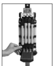
How to reposition a thruster: You'll notice that the bottom of each thruster is attached to a plastic anchor equipped with three flanges. Initially, the lowest of these three flanges is used to engage the thruster in the lower mount. Grip the anchor and disengage it by pulling outwards. Now, re-engage the anchor. Shift it down to the next-lowest flange and push it back into place.
