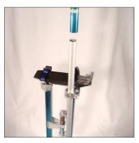
(6) Slide the *upper strut tubes* (H5) down over the *lower strut tubes* and through the *tube clamps*.
