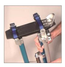
(3) Insert *lower strut tubes* (H23) up through the bottom of the *tube clamps*.
