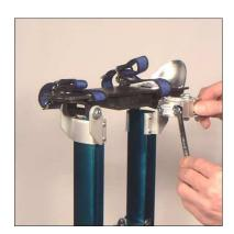
(2) Loosen the tube clamps (H29 / H30).
