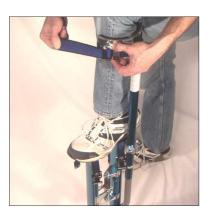
(1) IMPORTANT! Always buckle *leg straps* (H4) first, and then buckle *arch* (H7) and then *toe straps* (H8). When dismounting unbuckle the straps in reverse sequence.
