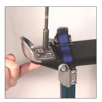
(1) The six holes in the *heel bracket* (H10) that is attached on the *footplate* (H9) are used to adjust the distance between the footplate and the heel bracket.
