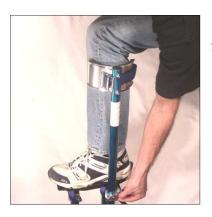
(7) Put your leg on the stilts and position so the *leg bands* (H4) are just above the large portion of the leg calves. Tighten the screws of the *tube clamps* well.
