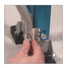
(5) Connection with attachment *cap screw* (H24) & *nylon lock nut* (H13A). Tighten well when assembly is complete.
